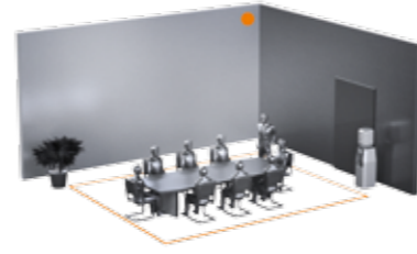
Conference-room situation, detection by the HPD2. Number of persons is detected.
