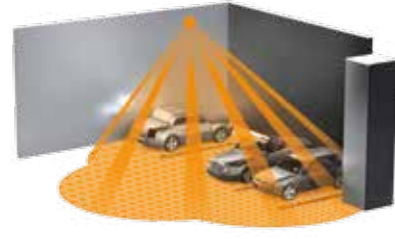
Multi-storey car park situation, detection by the IS 3360
