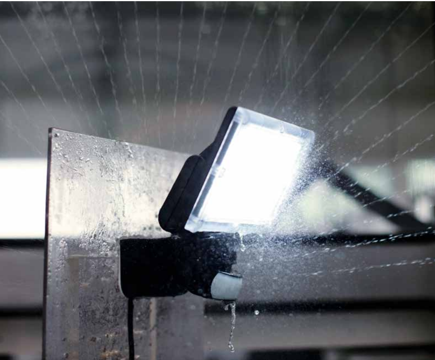
XLED home 1 put to the acid test: Our splashing-water test guarantees weather resistance and IP44 rating.
